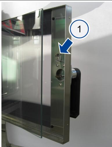
A photograph of a stainless steel door frame with a glass panel. A blue arrow points to a small circular button labeled '1' on the right side of the frame, which is the quick closure mechanism. |
