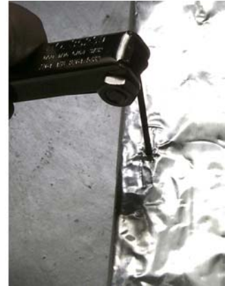
Fig. 19. Puncture foil with Allen wrench to loosen slot.
