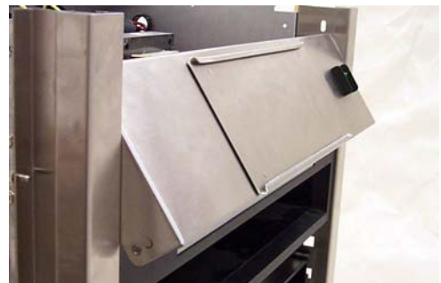
Fig. 3. Removing front fascia.
