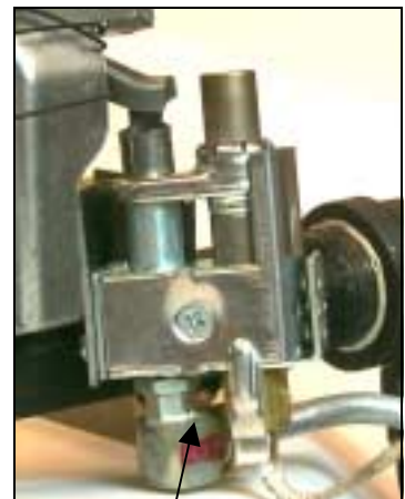
Clip used to remove thermopile.
